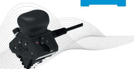
sg NDT wave probes are specially designed to perform handheld inspections of carbon steel and stainless-steel welds that have a rough surface finish. The probe is equipped with dynamic lift-off technology, which makes it ideal for inspecting painted or coated welds without having to remove and reinstate the coating. The probe's memory stores calibration data, making it easy to use and access when needed.
